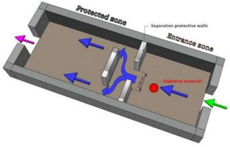
Figure 31: Example of a meandering wall. Source: Karlos and Larcher (2020).
