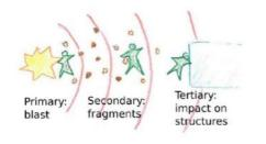
Figure 29: Hazards emanating from an explosion
