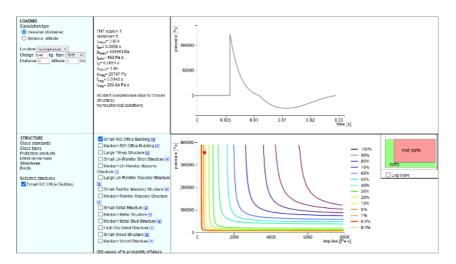
Figure 27: Example from the BIAssTool for the calculation of peak pressure / impulse parameters and comparison with pressure–impulse iso-damage curves
