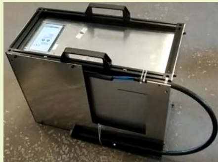
Portable spectrometer for detecting chemical precursors to explosives. ML for spectral analysis
